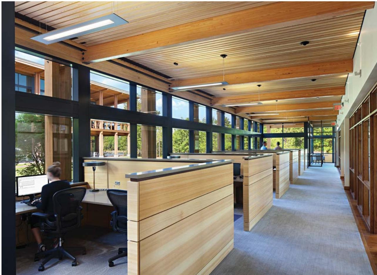
**CYPRESS PLYWOOD** was used to construct open-air work stations in the bank's new headquarters. It was also used on ceilings and beams.
